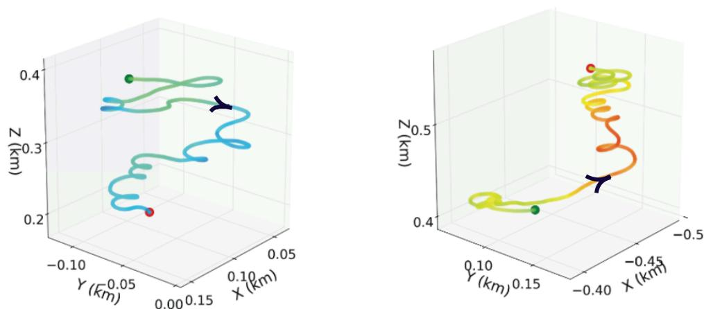
**Figure 16.10:** Sample thermal soaring trajectories, with arrows showing the direction of flight from the same starting point (note that the altitude scales are shifted). Left: before learning; the agent selects actions randomly and the glider descends. Right: after learning; the glider gains altitude by following a spiral trajectory. Adapted with permission from PNAS vol. 113(22), p. E4879, 2016, Reddy, Celani, Sejnowski, and Vergassola, Learning to Soar in Turbulent Environments.
