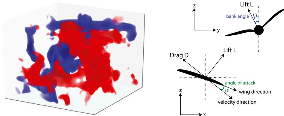
**Figure 16.9:** Thermal soaring model: Left: snapshot of the vertical velocity field of the simulated cube of air: in red (blue) is a region of large upward (downward) flow. Right: diagram of powerless flight showing bank angle  $\mu$  and angle of attack  $\alpha$ . Adapted with permission From PNAS vol. 113(22), p. E4879, 2016, Reddy, Celani, Sejnowski, and Vergassola, Learning to Soar in Turbulent Environments.
